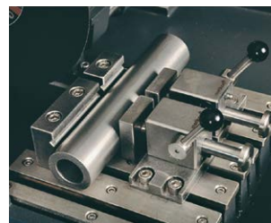
Stainless steel clamping devices and T-Slotted table
