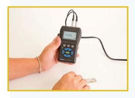
With more than 75 years of world-wide experience in ultrasonic design, Danatronics is pleased to welcome our EHC-03 to our corrosion thickness gage family. The EHC-03 is designed to accurately and non-destructively measure metal structures subject to corrosion.
