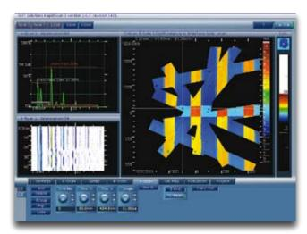
A common application for RapidScan2 is the inspection of carbon fibre composite components to detect delaminations and large voids. BVID (barely visible impact damage) is easily visualised, showing the full extent of the sub-surface defects. Detection and interpretation is simplest with time
